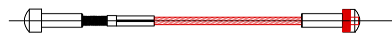
1:2 Jakob or similar 4mm Stainless steel rope system with stainless steel tension fixings
